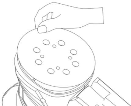
To install the abrasive disc, first remove all dirt or foreign matter from the pad. Then peel off the backing paper from the abrasive disc and attach the abrasive disc to the pad. Be careful to align the holes in the abrasive disc with those in the pad.
