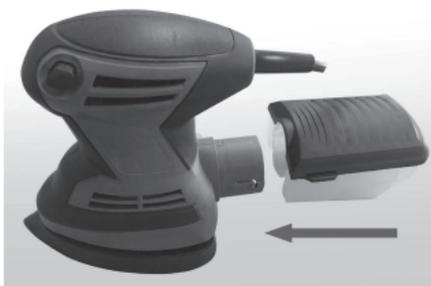
1. To install dust box, align the notches on both sides of dust bag with the buckles on both sides of dust port and push the dust bag completely onto place over the dust port on the back of the sander (Fig. 3).
