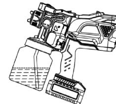
a) If spray in an upward direction, the angled end of the suction tube should be pointing toward the rear of the gun.
