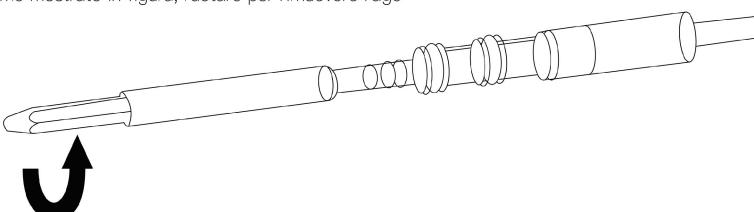
b) As shown in the figure, rotate to set up the needle
