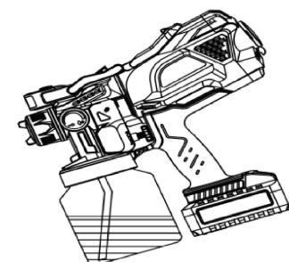
b) If spray in a downward direction, the angled end of the suction tube should be pointing towards the front of the gun.
