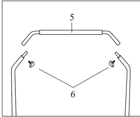
6. Make sure the bottom of the support pipe touch the floor steady. Then twist four triangular knobs(No.6) to the handlebar assembly.
