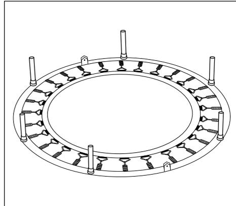
3. Remove a top rubber cap from a foot pipe. Skip a foot pipe to remove another rubber cap from the third one. Attach two support pipes(No.2) to these two foot pipes. Cover two caps back.
