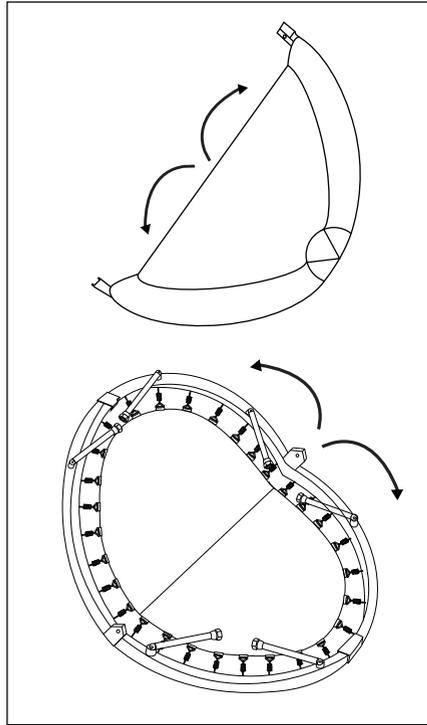
2. Pull six leg pipes up and then insert them into the socket of the frame.
