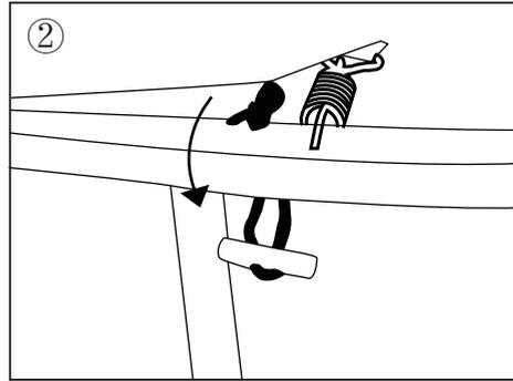
**Attention:** If you want to fold the jumping frame, you MUST take off the spring pad firstly. Otherwise, the spring pad will be damaged.
