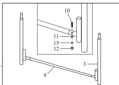
5. Insert two leg pipes to two bottom extension pipe assemblies. Put the frame on the them. Screw those two leg pipes to the frame.
