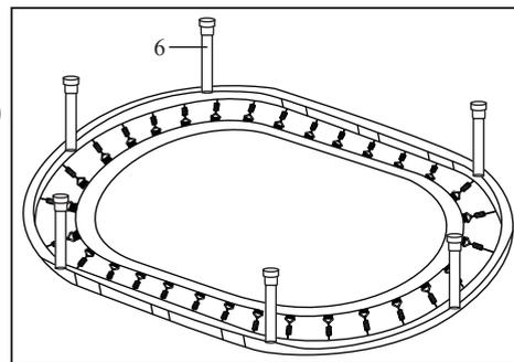
4. Connect two extension pipe assemblies (No.3) with the stabilizer bar(No.4). Insert a M6\*35mm bolt(No.10) to one side of the stabilizer bar. Then screw a washer (No.11), a split washer(No.15) and a lock nut(No.12) to fix. Please don't fix the another side of the stabilizer bar before you finish the Step 5.
