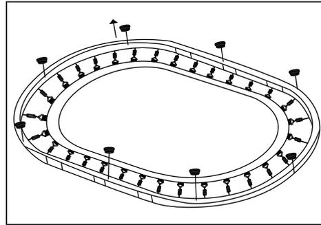
3. Screw six leg pipes(No.6) to the frame. (Don't screw them to two middle holes now, if you want to assemble the handrail finally.)
