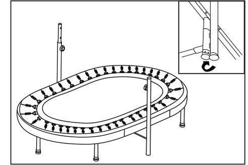
6. Insert a pipe holder bracket(No.9) into the gap between the extension pipe assembly and the frame. Insert two carriage bolts(No.14) and attach a pipe clamp(No.8).Screw two washers(No.11), two split washer(No.15)and two lock nuts (No.12) to fix them. (The other side is in the same way.)
