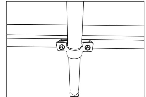
7. Adjust the height of two extension pipes to the top level. Assemble the handrail(No.5) to the extension pipe assemblies. Screw two triangular head bolts(No.13) to fix.
